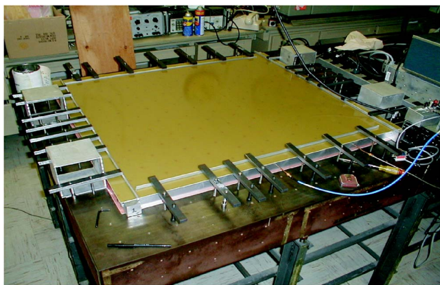
FIG. 4. (Color online) Photograph of our experimental setup. The four aluminum bars put on the top lid to help prevent lid buckling (see Sec. VI D) were removed for the photograph. Note the thin aluminum strips. They direct the downward force of the steel clamps to make good electrical contact between the copper-coated circuit board and the inside edge of each side-wall bar.
